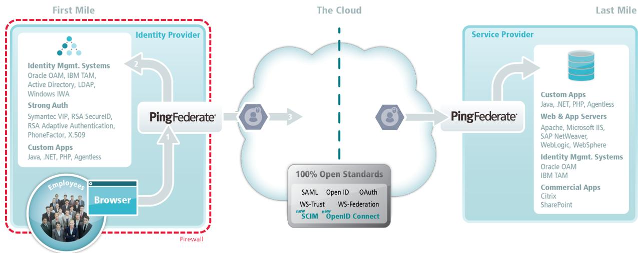
**Figure 3: Multiple security-domain, multi-protocol federation**
